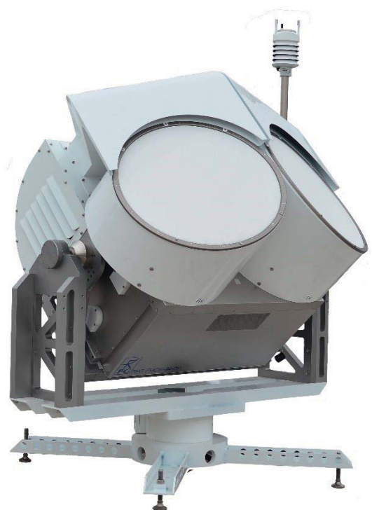
Fig. 8. The W-band cloud radar with the scanning unit.
